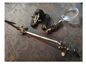
Separate all parts of the «third hand». Keep the articulations which will be used to fix the spindle to the macrophotography rail upper support. If the screws are to short for a good fixation, just use longer screws. Congratulations, you have built
