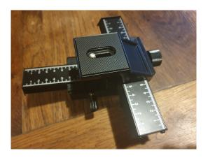
Turn the rail over and separate the two sliders. (a simple screw to unscrew)
