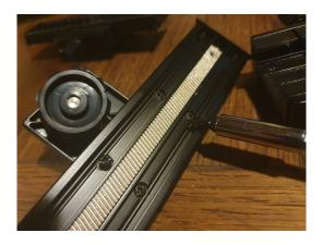
You can remove the the upper support if you want a longer winder. In that case you'll just use the screw to fix one slider above the other one.
