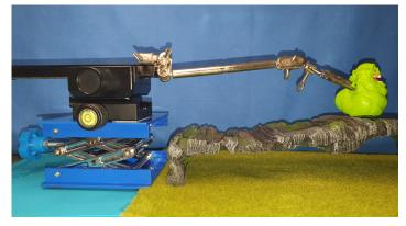
The complete set in two configirations: on left with the upper support, and on right with the slider without support. Note that in the configuration with above support, as this one is fixed on the middle of the rail, the working distance is half (5 cm) of the config without it (10 cm).
