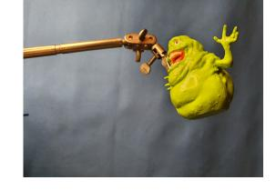
The elevator allows to place subjects «in the air» and you now can move them very precisely in both 2 dimensions.
